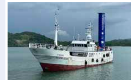
▲ The bound4blue eSail in operation on the fishing vessel Balueiro Segundo in June 2021. Image: bound4blue
