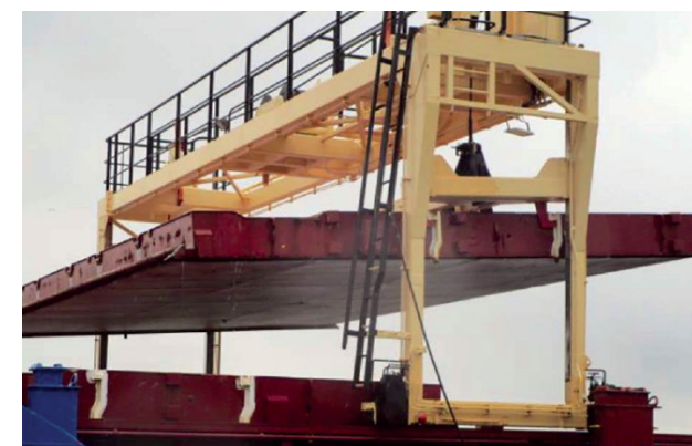
▲ Cimbris gantry crane with hatch cover suspended
