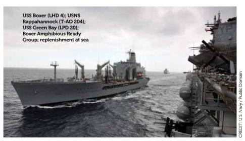
B. It's very dynamic and requires an understanding of the situations like sailing right alongside a vessel at 150 feet at 12 or 13 knots while pumping very volatile diesel and jet fuel over to them.
